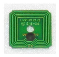
The Escort Memory Systems LRP family of RFID tags provides outstanding auto-ID solutions for demanding industrial environments. The "i" tag is based on a one kilobyte memory chip and incorporates EMS' unique design and manufacturing technology. The tag requires no batteries.
